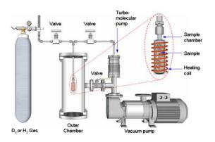
FIGURE 2. Schematic of the gas-loading system.
